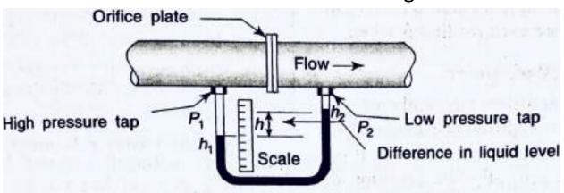
Working When there is a pressure difference between the two ends of the tube, the liquid level goes down on one side of the tube and up on the other side. The difference in liquid levels from one side to the other indicates the difference in pressure. From the above figure, the differential pressure ( $P_1 - P_2$ ) is obtained by the relation:
