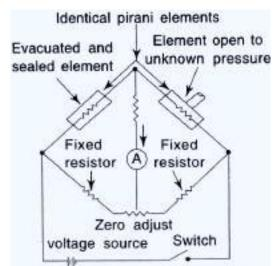
evacuated glass, while the other filament is kept in a container connected to the source of pressure.
