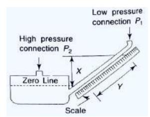
expand the scale and thereby to increase the sensitivity even more. The inclined manometer is used to mea sure very small pressure differences (in hundredth of an inch of water). The distance y that the liquid moves through the tube is greater than the distance x that the liquid rises.
