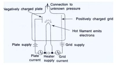
Any positively charged ions produced due to collision of electrons with gas molecules are attracted to wards the negatively charged plate.
