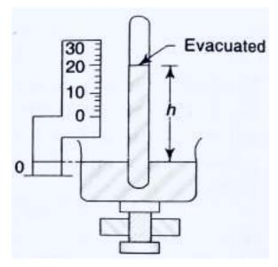
pressure. This is the principle of the barometer, as shown in figure. A barometer is a well-type absolute pressure gauge whose pressure range is from zero absolute to atmospheric pressure. Its readings are generally in millimeters of mercury (mm Hg). With a barometer, high vacuum is not measured. The pressure in the evacuated portion of the barometer is not really absolute zero but rather the vapour pressure of the filling fluid, mercury, at ambient temperature.
