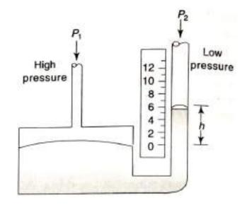
very small-sized tube. Thus the zero level moves very little when pressure is applied. Even this small error is compensated by suitably distorting the length of scale. However, such an arrangement is sensitive to nonuniformity of the tube crosssectional area and is thus considered some what less accurate. Figure shows a welltype manometer. In a single-leg instrument, high accuracy is achieved by setting the zero level of the well at the zero level of the scale before each reading is taken.
