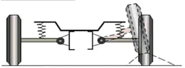
In this type of suspension system, both left and right wheels are connected to the axle via different links. This arrangement eliminates the effect of one wheel on the other. I other words, when a wheel rolls over a bump, it doesn't cause the other wheel to tilt.
