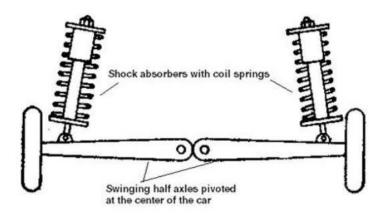
Both wheels are mounted rigidly on the half axles which are pivoted at the other end to the chassis member at the centre of the vehicle. The spring with the shock absorber is mounted on the half axle. Now when one wheel experiences a road shock, the axles attached to the wheel moves up and down without affecting the other wheel. The major disadvantage of this system is that:
