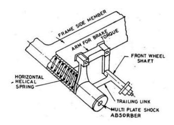
It consists of a horizontal torsion spring with shock absorber which is attached to a trailing link. The trailing link is attached to a shaft that carries the wheel hub. The other end of the torsion spring is attached to the frame side member. Now when the wheel moves up or and down, the spring winds and unwinds respectively. In some automobiles, torsion bars are used in place of automobiles. The major disadvantages of this system is:
