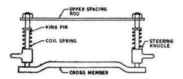
It consists of an extended cross member to which king pin of the stub axle is attached at one end. The coil spring and the shock absorber are attached on this stub axle. The other end of king pin is fixed to an upper spacing bar. According to the up and down motion of the wheel, the king pin is also allowed to move up and down thus compressing and elongating the spring. Major disadvantage of this system is decreased stability of the automobile.
