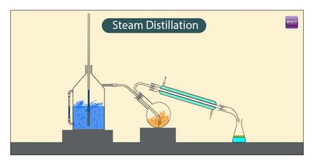
At a very high sustained temperature, few of <u>organic compounds</u> may decompose. It would be difficult to separate by a distillation process at a certain boiling point. Steam will be introduced into an apparatus (distillation).
