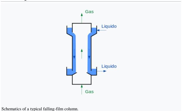
In the most common case, the column contains one liquid stream and one gas stream. The liquid forms a thin film that covers the inner surface of the vessel, [1] instead the gas stream is normally injected from the bottom of the column, so the two fluids are subjected to a countercurrent exchange of matter and heat, that happens in correspondence of the gas-liquid interface.
