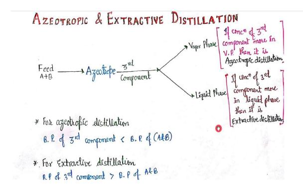
What is difference between azeotropic distillation and extractive distillation?
