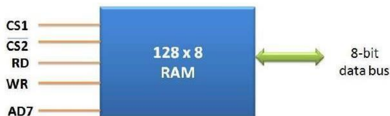
Block Diagram Representing 128 x 8 RAM (Random Access Memory)
