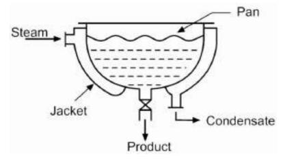
jacket is welded to the pan. The jacket is provided with a steam inlet at the top, while a condensate drain is provided at its bottom. The pan is provided with an outlet at the bottom for draining its contents. The jacket is usually constructed out of mild steel, while the pan is constructed out of mild steel, stainless steel, copper or aluminium as per process requirements.
