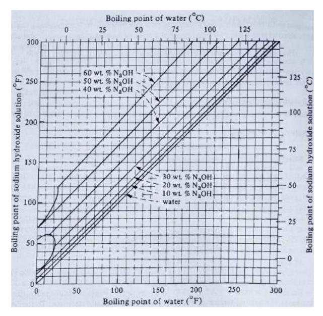
DÜHRING LINES FOR SOLUTIONS OF SODIUM HYDROXIDE
