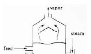
bundle at the lower portion of the shell. The horizontal bundle of heating tubes is similar to the bundle of tubes in a heat exchanger. A vapour outlet is provided on the top cover and a thick liquor outlet is provided at the bottom. Feed point is located at the left.
