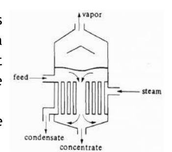
boiling liquid inside the tubes takes place from condensing steam the outside of tubes. Because of boiling and decreases in density, the liquid rises in the tubes by natural circulation and flows downward through a large, central open space or downcomer, where it is removed as a thick liquor. This natural circulation increases the heat transfer coefficient. The type of evaporator is not used with viscous liquids.
