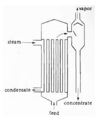
the ratio of feed to evaporation rate is low, natural recirculation of the product through the evaporator is effected by adding a large pipe connection between the outlet concentrate line and the feed line.
