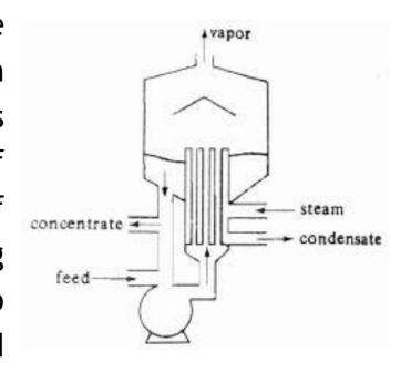
velocity of flow of liquor through tubes increases remarkably the liquid film heat transfer coefficients and the high velocity resulting by use of a centrifugal pump prevents the formation of excessive deposits on the heat transfer surfaces.
